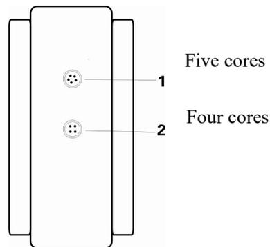
1, High voltage gun socket 2, Ground wire socket
