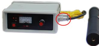
4、 Put the connecting magnet on the pipeline, and connect between long cable and the short connecting line, make sure the short connecting line have effective ground connection.
