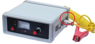
2、 open the host power: Tap the power switch, the power supply voltage indicator light, pointer meter display power supply voltage. The power supply voltage is less than 11V, timely charge before use. (When the main body charging, the charger is red, when fully charged, the charger becomes green).
